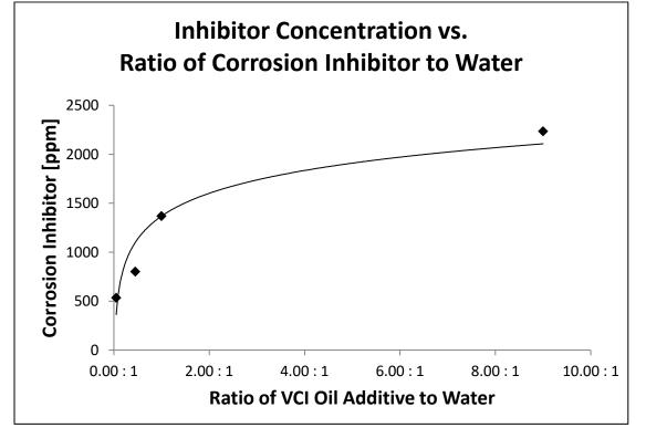
Figure 1: Corrosion inhibitor concentration compared to the ratio of VCI oil additive to water from extraction testing.
